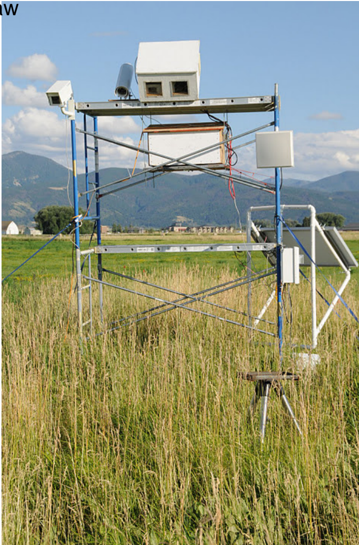
Multispectral imagers used to detect plant stress caused by CO 2 leaking from underground.
